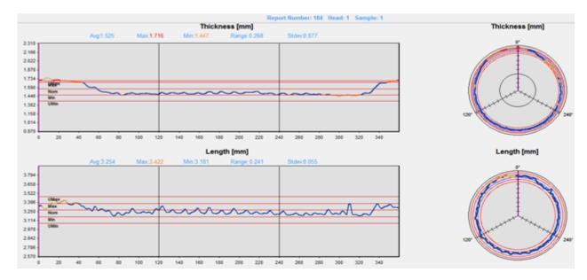
Sample SEAM360 report for 8x beverage cans each measured on only one side
