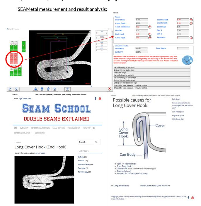
In above images, you see how the SEAMetal 6 software not only performs a measurement of the seam, there is also a SEAM analyse option. This option analyses the seam, and if somethings are out of specification, it provides information on what can be adjusted in the seamer.
