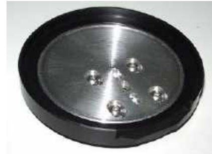
Separate chuck fit to be mounted on optical unit
