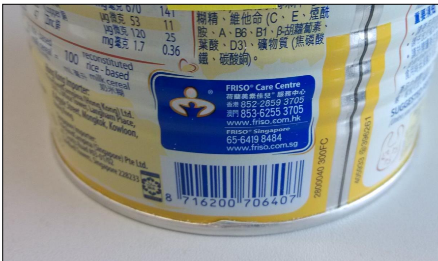
Above example images of infant formula can both the operator view and the actual can with a bad seam
