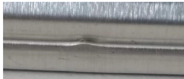
Above an example of a start-end seal fault that from top appears as a “dark spot”; rectangular fish can at its long straight side.
